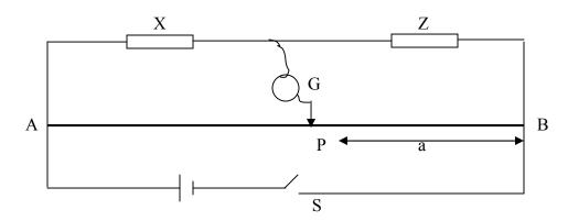
(f) Close the switch. Tap the jockey at various points along the wire AB and locate a point P at which the galvanometer shows zero deflection. Measure and record in the table below the length 'a' where a = PB
