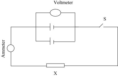
(b) With the switch open, record the reading E of the voltmeter
