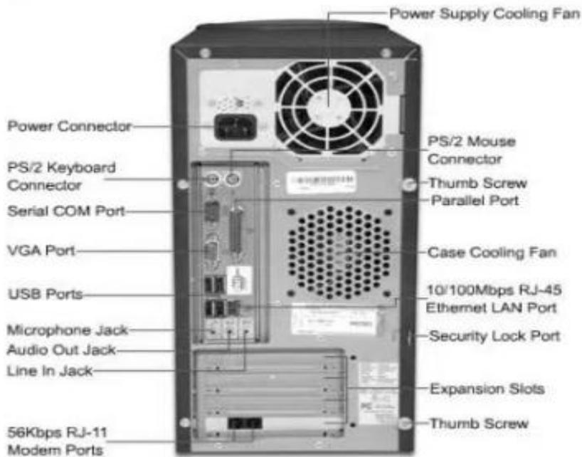
FIGURE 9: PORTS AND SOCKETS BEHIND THE CHASSIS
